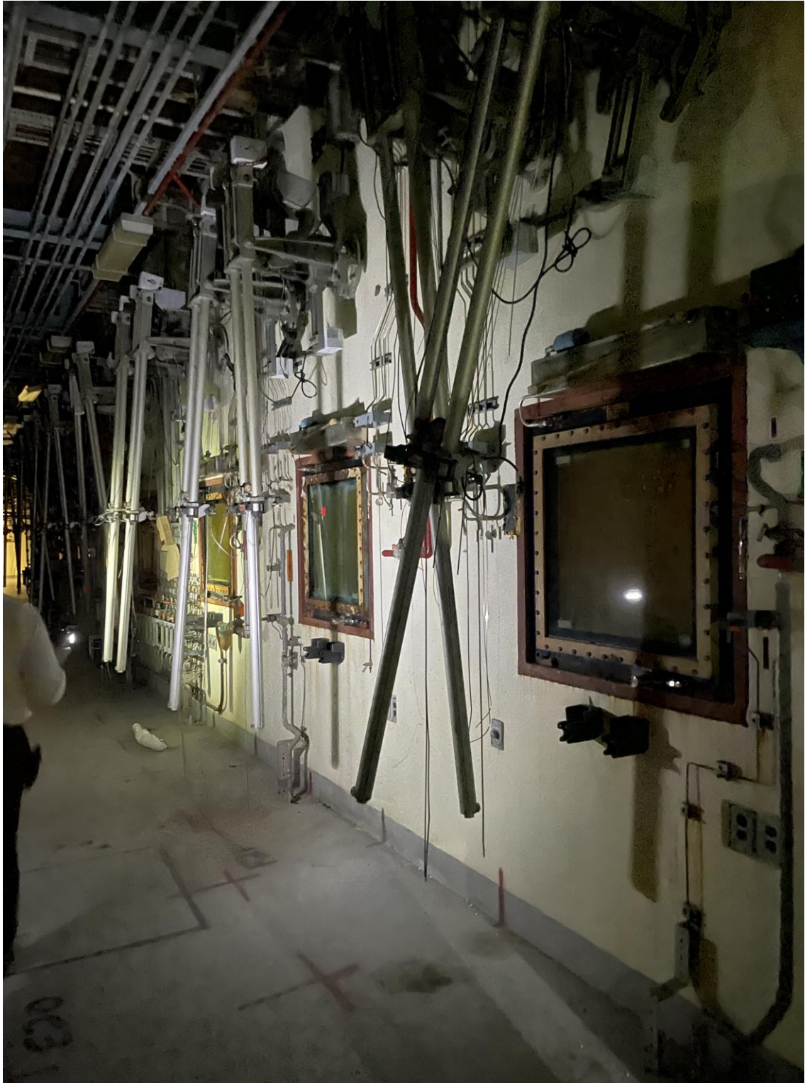
Hot boxes with mineral oil filled windows and old hand manipulators
