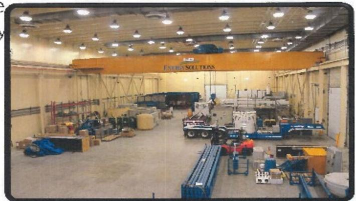
Building 201, the biggest asset we have there is the size of it for one, we have the 80 ton overhead crane which allows us to do a lot of special projects in there; that's also where our de-watering and cask maintenance is performed, in that building.
